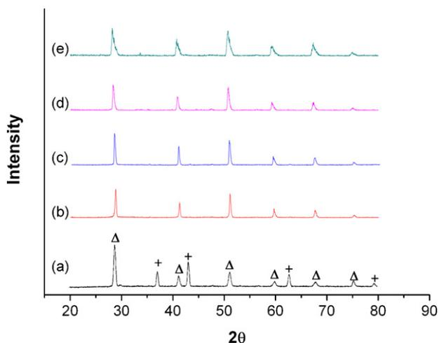
Fig. 4. XRD patterns for the bi-layers of (a) NiO–BCTY10 anode substrate, (b) BCTY10 membrane, (c) BCTY10 membrane after being boiled in water, (d) BCTY10 membrane after exposure to 100% CO<sub>2</sub> at 700 °C, (e) BCTY10 membrane after exposure to 100% CO<sub>2</sub> at 900 °C. (Δ) BCTY10; (+) NiO.
