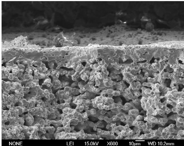
Fig. 6. SEM cross-sectional view of the single cell after testing.
