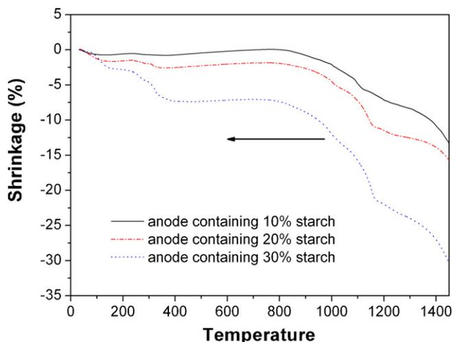
Fig. 1. Shrinkage of green anode substrates containing different amounts of starch.
