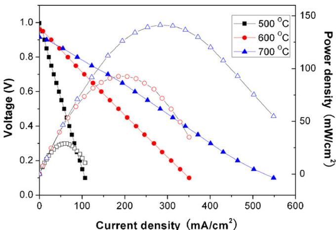
Fig. 7. Performance of a fuel cell with humidified hydrogen measured from 500 to 700  $^{\circ}\text{C}$ .
