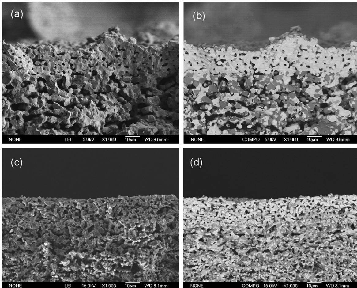
Fig. 3. Secondary electron image (a) and backscattered electron image (b) of the BCTY10 membrane on an anode substrate containing 30 wt.% starch after sintering at 1400 °C. Secondary electron image (c) and backscattered electron image (d) of the BCTY10 membrane on the 30 wt.% starch containing anode prepared by conventional powder solid state reaction after sintering at 1450 °C.
