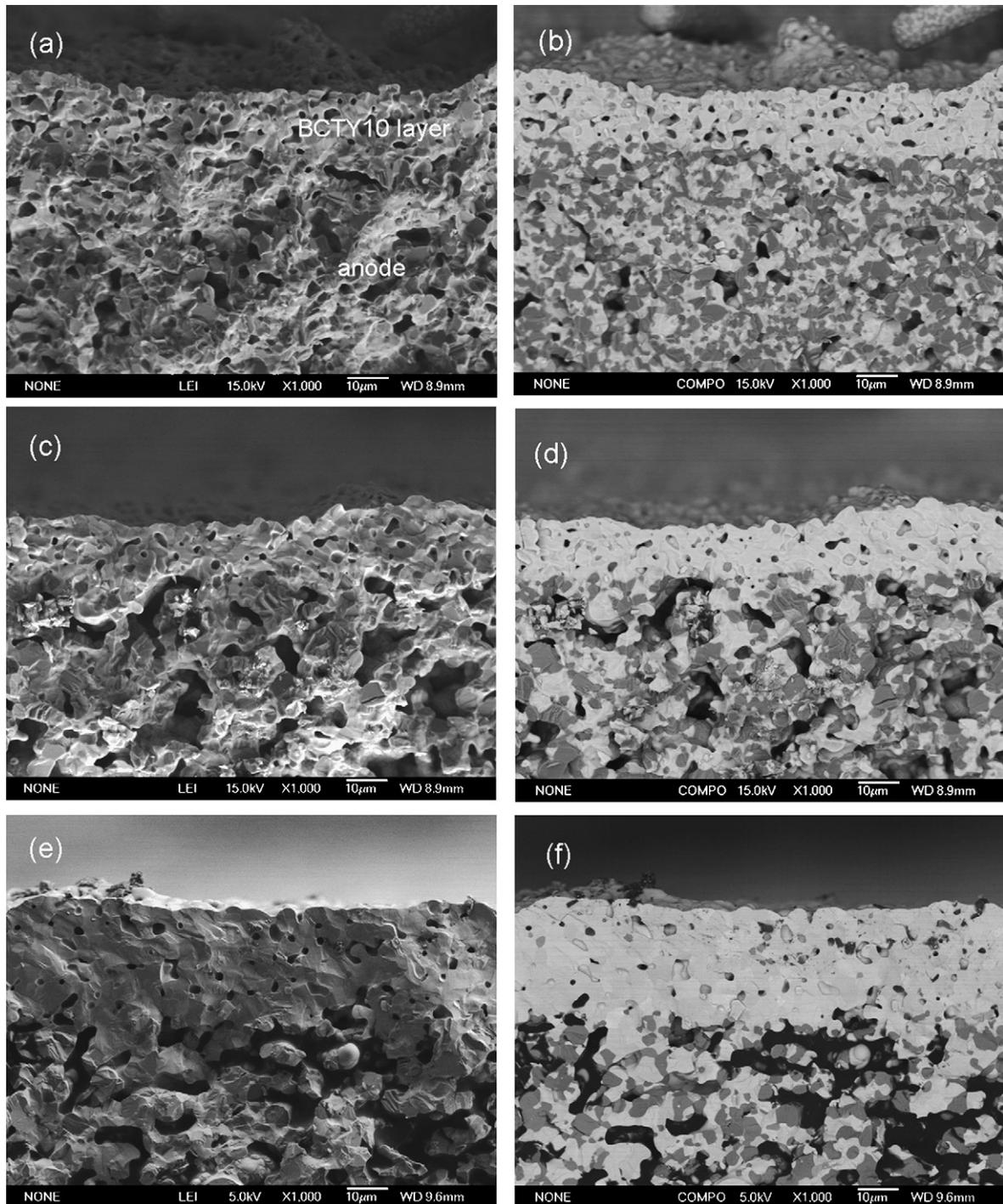
Fig. 2. Fracture surface of the half-cell based on a BCTY10 electrolyte membrane after sintering at 1450 °C. Secondary electron images of BCTY10 membranes on the anode substrates containing different amounts of starch (a) 10 wt.%, (c) 20 wt.% and (e) 30 wt.%. Backscattered electron images of the corresponding areas for (b) 10 wt.% starch containing anode, (d) 20 wt.% starch containing anode and (f) 30 wt.% starch containing anode.
