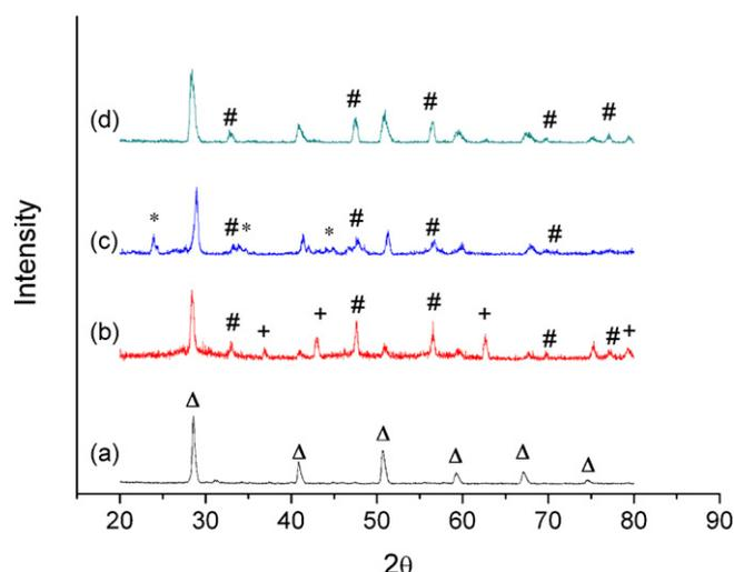
Fig. 5. XRD patterns of (a) BZCY7 membrane, (b) BZCY7 membrane after being boiled in water, (c) BZCY7 membrane after exposure to 100% CO<sub>2</sub> at 700 °C, (d) BZCY7 membrane after exposure to 100% CO<sub>2</sub> at 900 °C. (Δ) BZCY7; (+) NiO; (#) CeO<sub>2</sub>; (\*) BaCO<sub>3</sub>.
