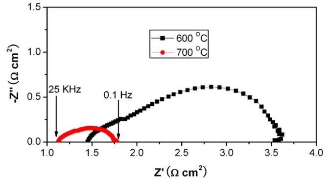
Fig. 8. Impedance spectra of a single cell measured under open circuit conditions at different temperatures.
